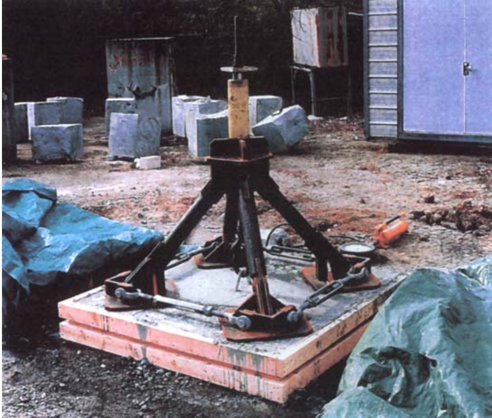
Photo 4. Load frame, ram, and jack
