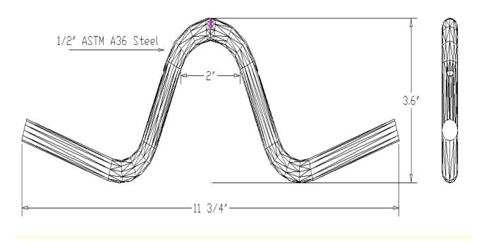
Load ratings were established when anchors were installed in recess pockets so that the top of anchor is 34 " recessed from concrete surface.\*
