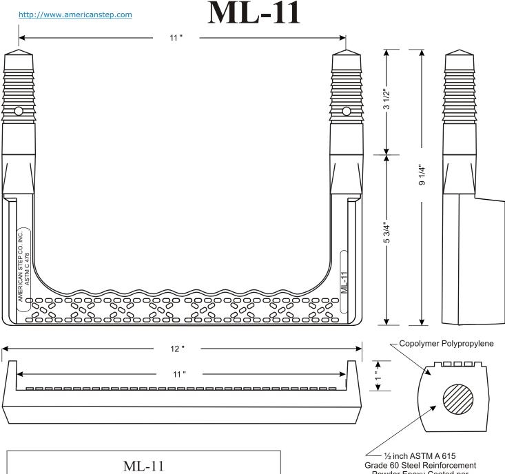
Mechanical Lock Installation Methods Minimum Concrete Strength Must Be 3000 psi.
